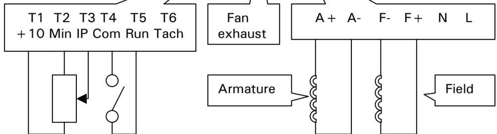
**Earthing** The terminals are non-isolated hence do not earth. The motor earth should be connected to the system enclosure earth.
