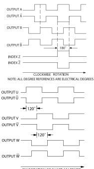
CW ROTATION OF SHAFT AS VIEWED LOOKING AT THE ENCODER FACE. NOTE: ALL DEGREE REFERENCES ARE ELECTRICAL DEGREES.
